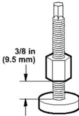
**STEP 3.** Screw leg into washer base by hand until nut reaches washer base. Repeat for other leg.
