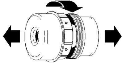
**STEP 3.** Remove internal holding cup.
