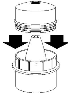
**STEP 7.** Replace the dispenser on the agitator; press firmly to snap into place.
