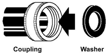
**STEP 1.** Insert one new, flat washer (from the parts bag) into each end of the inlet hoses. Check that washers are firmly seated in couplings.
