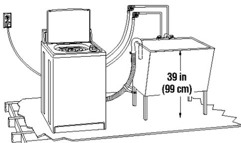
Standpipe Drain System (p. 13)
