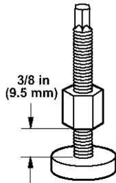
**STEP 3.** Screw leg into washer base by hand until nut reaches washer base. Repeat for other leg.
