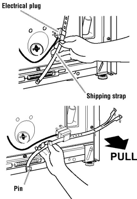
**STEP 2.** Pull firmly to remove the end of the shipping strap that remains pinned to the back of the washer. This will release the rear self-leveling legs.
