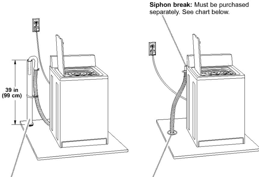
**Standpipe drain system:** Needs a 2-in (5 cm) minimum diameter standpipe with minimum carry-away capacity of 17 gal (64 L) per minute. Top of standpipe must be at least 39 in (99 cm) above floor and no higher than 96 in (2.4 m) from bottom of washer.
