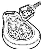
**Dissolves powder or liquid detergents before applying to load. When desired add powder or liquid color safe bleach to this dispenser.**
