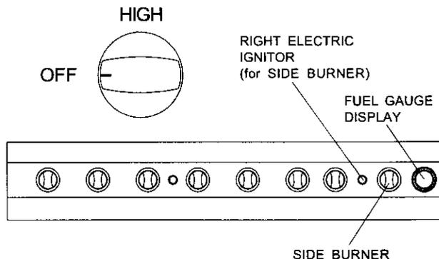
3. Immediately press the electric ignitor for 3-4 seconds to light the burner.
