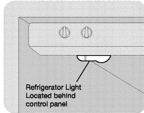
Refrigerator Light Located behind control panel
