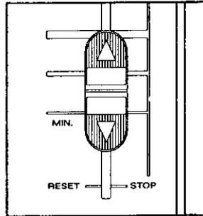
Next, slowly slide the speed control up until the walking belt begins to move at slow speed. Carefully step onto the walking belt and begin walking. Change the speed of the walking belt as desired by sliding the speed control.
