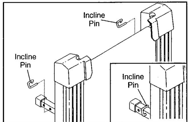
**CAUTION: Before using the treadmill, make sure that both incline legs are at the same height. Do not use the treadmill with the incline pins removed.** After you have adjusted the incline legs, lower the treadmill (see HOW TO LOWER THE TREADMILL FOR USE on page 11).
