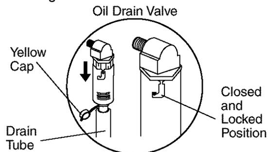
3. Unlock drain valve by pushing upward slightly and turning counterclockwise.
