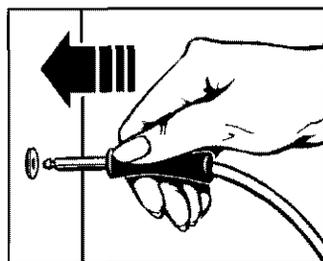
**Step 1:** Insert probe in food as directed in the Cooking by Temperature section. Plug other end of probe securely into wall receptacle.
