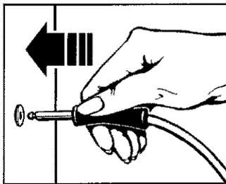
**Step 1:** Insert the temperature probe into food as directed in the Cooking by Temperature section. Plug the other end securely into the oven wall receptacle.
