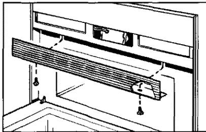
**Step 3:** Rotate the light bulb housing out and toward you to access the light bulb. Replace the burned-out bulb with a 40-watt incandescent bulb (WB02X4253) available from your GE supplier.
