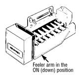
The icemaker will fill with water when it cools to freezing. A newly-installed refrigerator may take 8 to 12 hours to begin making ice cubes.
