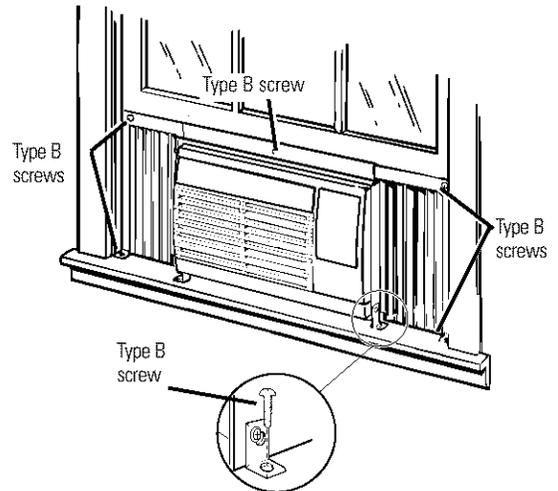
Attach the brackets to the stool on both sides using two type B screws.
