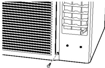
On some models, remove the bottom right grille screw.
