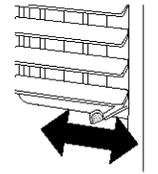
To open the vent, push the lever to the right.
