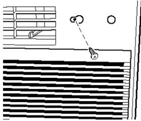
On some models, remove the knobs, filter and screw behind the filter bottom.
