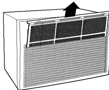
Grab the tabs on the filter and pull it up and out.
