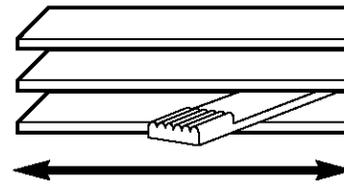
To open the vent, push the lever to the right.
