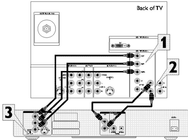
**1** Connect from the YPrPb jacks on the back of the DVD player to the HD INPUT-AV 4 G/Y, R/Pr, B/Pb jacks on the back of the TV.
