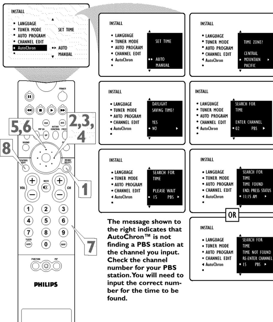
The message shown to the right indicates that **AutoChron™** is not finding a **PBS** station at the channel you input. Check the channel number for your **PBS** station. You will need to input the correct number for the time to be found.
