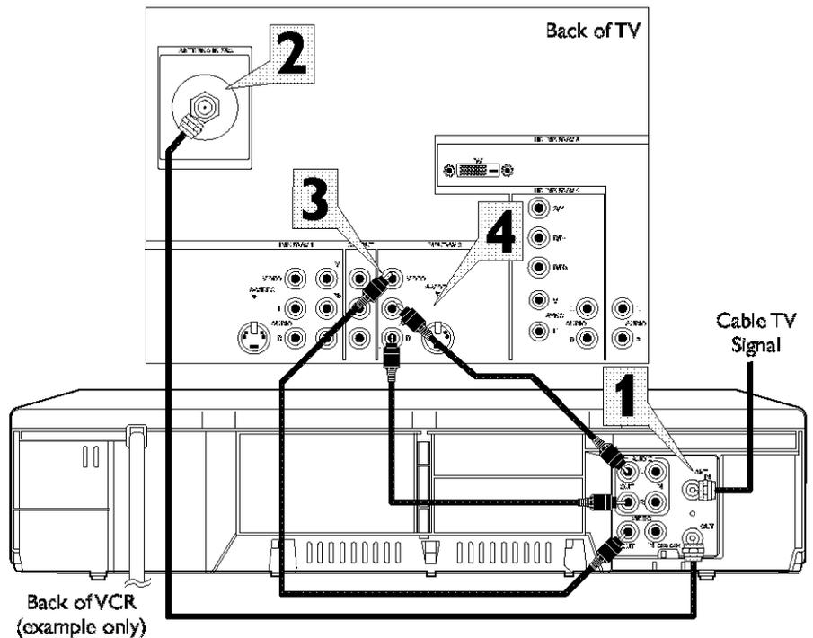
**1** Connect a cable TV or antenna signal to the ANT IN jack on the back of the VCR.
