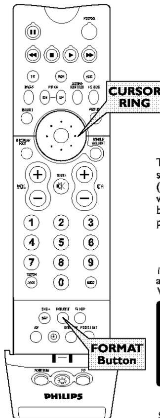
The picture-format modes are available for use only with video sources connected to the ANTENNA, AV1, CVI, AV2, and AV3 (Side Panel) inputs on the TV. Control the picture formats of video sources connected to the HD inputs through the set-top box (for HD programming) or progressive-scan-capable DVD player (for DVD programs)
