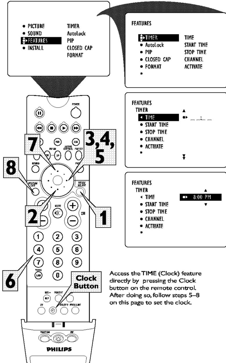
Access the TIME (Clock) feature directly by pressing the Clock button on the remote control. After doing so, follow steps 5–8 on this page to set the clock.
