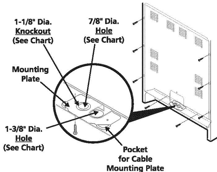
**NOTE:** Range is shipped from factory with 1-3/8" dia. hole as shown. To use either 7/8" dia. hole or 1-1/8" dia. knockouts:
