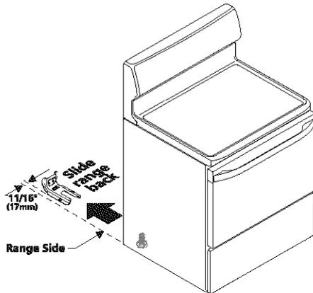
Visually check that rear leveling leg is inserted into and fully secured by the Anti-Tip Bracket by removing lower panel or storage drawer. For models with a warmer drawer or broiler compartment, grasp the top rear edge of the range and carefully attempt to tilt it forward.
