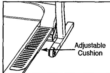
the cushions to level 2 or 1. It may be helpful to lift on the walking platform as you rotate the cushion. **Note: The faster you run on the treadmill, or the heavier your weight, the firmer the cushioning system should be. Make sure that both cushions are at the same setting.**
