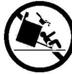
**⚠ WARNING** To reduce the risk of tipping, the range must be secured by properly installed anti-tip bracket provided with the range. To check if the bracket is installed properly, grasp the top rear edge of the range and carefully attempt to tilt it forward. Refer to the Installation Instructions for proper anti-tip bracket installation.
