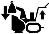
Weight Transfer Lift Handle To Engage
