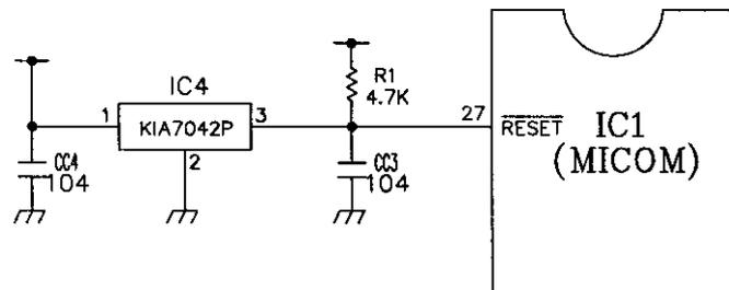
The RESET circuit is for allowing all the functions to start at the initial conditions by initializing various parts including the RAM inside the MICOM (IC1) when the power is initially supplied or the power supply to the MICOM is restored after a momentary power failure. For the initial 10ms of power supply, LOW voltage is applied to the MICOM RESET terminal. During a normal operation, 5V is applied to the RESET terminal. (If trouble occurs in the RESET IC, the MICOM will not work.)
