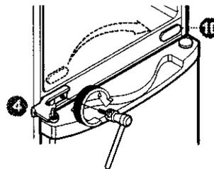
**9** Reassemble the refrigerator door stopper **11**.
