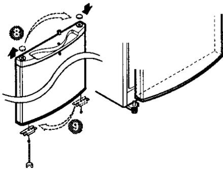
**8** Move the cap **10** and reassemble the center hinge **4** after removing the washer.
