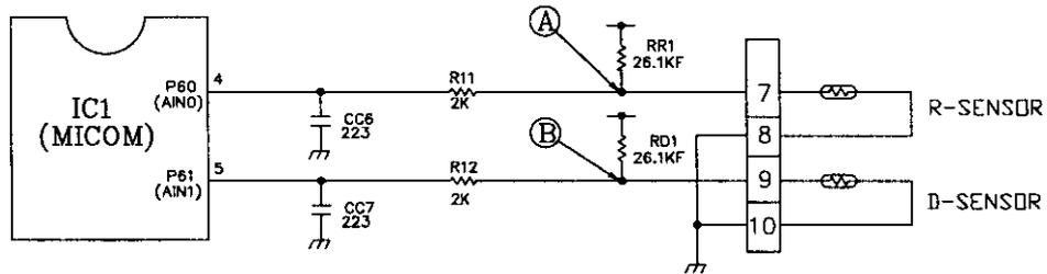
The upper CIRCUIT reads REFRIGERATOR temperature and Defrost-Sensor temperature for defrosting into MICOM. OPENING or SHORT state of each TEMPERATURE SENSOR are as follows.
