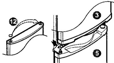
**11** Move the pin position **13** of the upper hinge.
