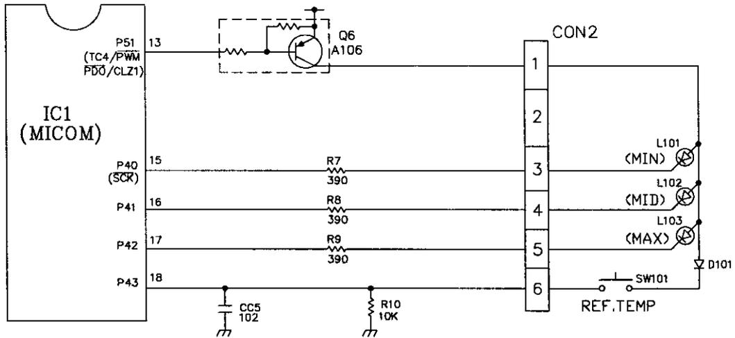
◆ The circuit shown above is to determine whether a function control key on the operation display is pushed and to turn on the corresponding function indication LED. The drive type is the scan type.
