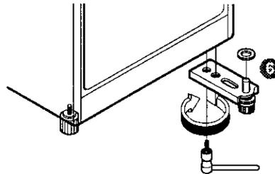
**5** Reposition the adjustable screw assembly **7**.
