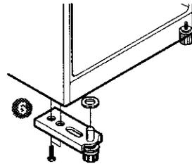
**7** Move the cap **8** and bracket **7** of the refrigerator door.
