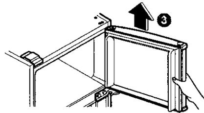
**3** Separating the center hinge ④ and the refrigerator door ⑤.
