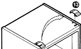
**12** Assemble the upper hinge **2** and the cap **1**.
