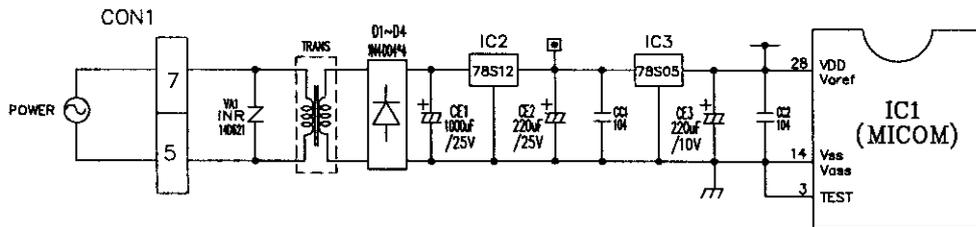
The secondary part of the TRANSFORMER includes the power supply for the display and the relay drive (12 Vdc) and the power supply for the microprocessor and IC (5 Vdc.)
