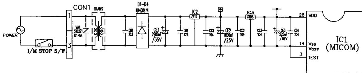
The secondary party of transformer consists of power (12Vdc) for driving display and relay and power (5Vdc) supplying power to MICOM and IC.
