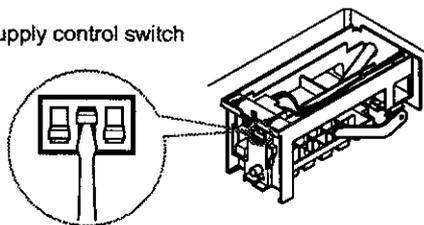
\* Adjust the water supply control switch to adjust the amount of water being supplied.
