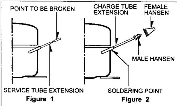
It is necessary to execute the soldering operation with valve open so that the fumes caused by oil residue can come out freely without blowholes between two tubes during the heating the of the point to be soldered.
