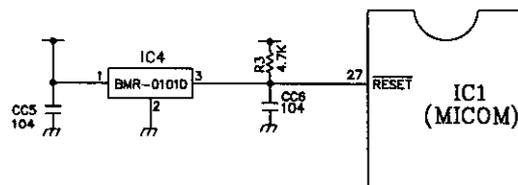
The reset circuit is a circuit that initializes various parts such as RAM, etc inside of the MICOM (IC1) and starts the whole of function from the initial status and 'low' voltage is applied for a constant time (10ms) at the reset terminal of the MICOM at the start of power input.
