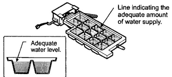
\* Make sure it is adjusted to meet the line indicating the adequate amount of water supply.
