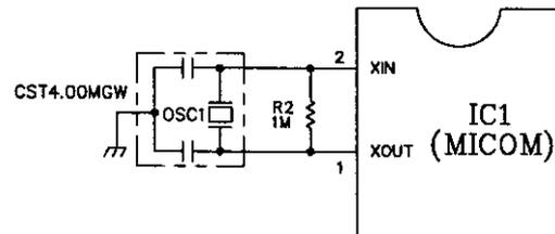
Circuit used for synchronous clock generation for transmitting/receiving information of the inside logic elements of IC and basic time generation for calculating time. Rated parts must be used as counting time is changed at the IC1 or the OSC1 does not operate if SPEC would be changed.
