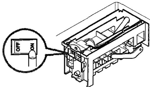
\* Make sure the switch on the ice maker assy is turned "on".
