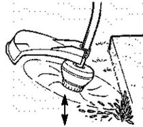
**SCALPING** – The scalping technique removes unwanted vegetation down to the ground. Hold the bottom of the trimmer head about 3 in. (8 cm) above the ground and at an angle. Allow the tip of the line to strike the ground around trees, posts, monuments, etc. This technique increases line wear.
