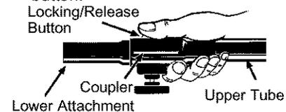
3. While securely holding the engine and upper tube, pull the attachment straight out of the coupler.
