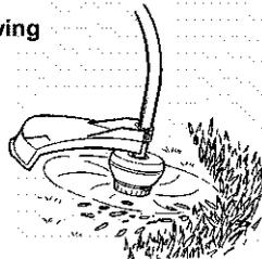
**SWEEPING** – The fanning action of the rotating line can be used to blow away loose debris from an area. Keep the line parallel to and above the area surface and swing the tool from side to side.
