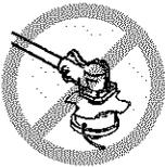
**⚠ WARNING:** The blade continues to spin after the throttle is released or engine is turned off. The coasting blade can throw objects or seriously cut you if accidentally touched. Stop the blade by contacting the left hand side of the coasting blade with material already cut.
