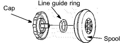
Use a pre-wound spool or refill spool with line. If using a pre-wound spool, remove tape strip from line and spool.
