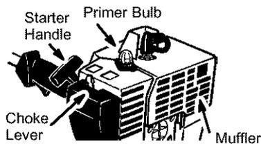
6. Pull starter rope handle sharply until engine sounds as if it is trying to start, but do not pull rope more than 6 times.
