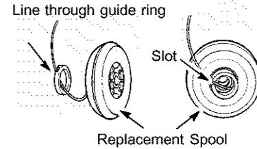
3. Rest guide ring on spool and place line through slot. Allow line to extend 4 - 6 inches (10 - 15 cm) from center of spool.
