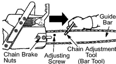
2. Loosen chain brake nuts until they are finger tight against the chain brake.
