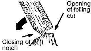
**NOTE:** Before felling cut is complete, use wedges to open the cut when necessary to control the direction of fall. Use wood or plastic wedges, but never steel or iron, to avoid kickback and chain damage.
