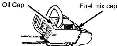
oils will cause engine damage. When mixing fuel follow the instructions printed on the container. Always read and follow the safety rules relating to fuel before fueling your unit.
