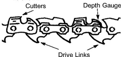
8. Place chain over and behind clutch, fitting the drive links in the clutch drum sprocket.
