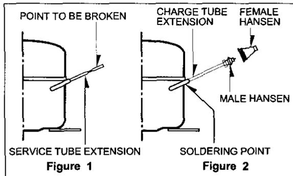
It is necessary to execute the soldering operation with valve open so that the fumes caused by oil residue can come out freely without blowholes between two tubes during the heating of the point to be soldered. The extension fitted with the male Hansen is connected to the female fitting of the vacuum pump tube. (Figure 3)
