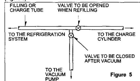
In addition, check the graduated scale on the cylinder for the quantity of R-134a to be added, for example, if we have 750 grams of Freon in the cylinder and must add 140 grams to the group, this amount will be reached when R-134a has dropped to 610 grams, remembering that the indicator shows a lower limit of meniscus. Do this after choosing the scale corresponding to the gas pressure different scales reported as the same gas pressure indicated by the pressure gauge on the top of the column.
