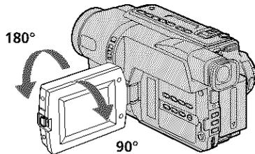
When closing the LCD panel, set it vertically until it clicks, and swing it into the camcorder body.
