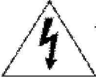
The lightning flash with arrowhead symbol within an equilateral triangle is intended to alert the user of the presence of uninsulated "dangerous voltage" within the product's enclosure that may be sufficient magnitude to constitute a risk of electric shock.
