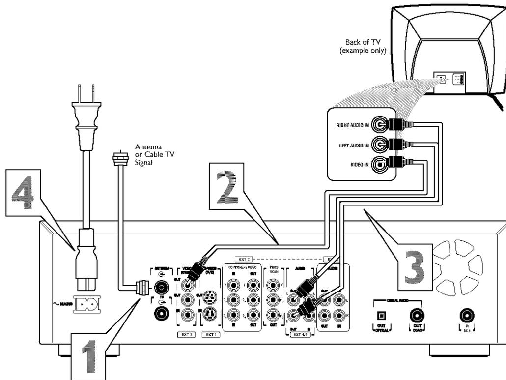
**1** Connect your Antenna or Cable TV signal to the ANTENNA jack on the rear of the DVD Recorder.
