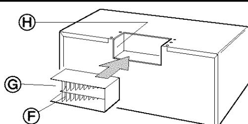
Slide air deflector back into cabinet as far as it will go. Check that deflector vanes ® face the rear of the cabinet and that the small exhaust ports © ® face each other.
