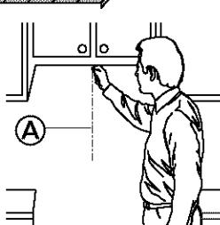
Using measuring tape, find and clearly mark the vertical centerline **A** of the cabinet opening on the wall directly under the upper cabinet.
