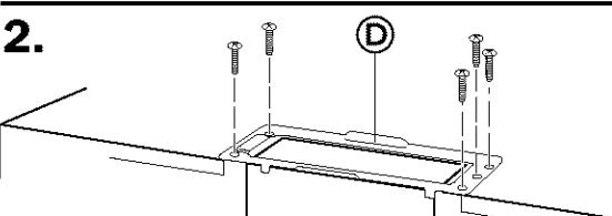
Remove 5 screws that attach damper plate © to top of microwave hood cabinet.
