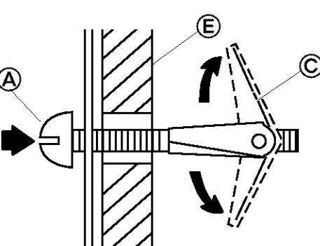
Finger tighten the toggle bolts **A** to make sure toggle nuts **C** have opened against drywall **E**.
