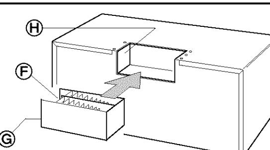
Slide air deflector back into cabinet as far as it will go. Check that deflector vanes ® face the top of the cabinet and that the small exhaust ports © ® face each other.
