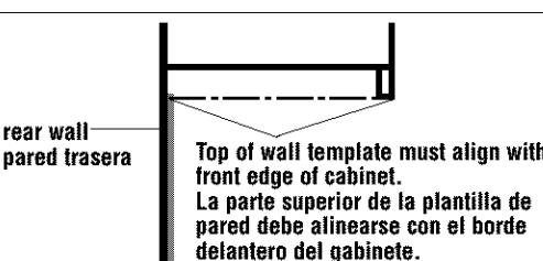
Line up paper wall template centerline with centerline on wall. Tape or tack wall template to wall. Top of template must be located a minimum of 66" from floor.
