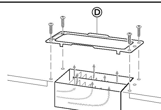
Reattach damper plate © with four screws at each corner of the damper plate. Save bright-colored tapping screw for use later to attach damper assembly.
