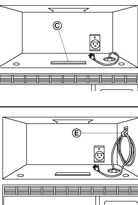
Coil power supply cord through clamp **E**. Secure clamp to cabinet side wall with dark colored screw.
