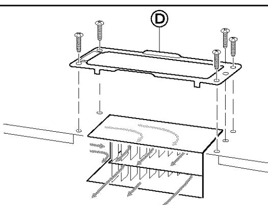
Reattach damper plate © with five screws.
