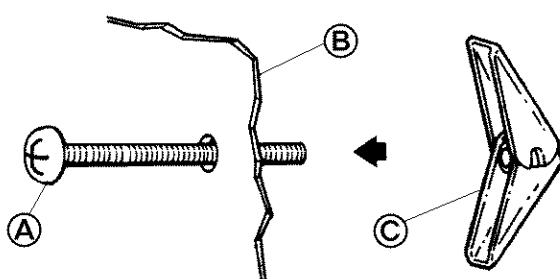
Insert 1/4-20 x 3" toggle bolts **A** through holes in mounting plate **B** that match the location of the 3/4" holes in the drywall.
