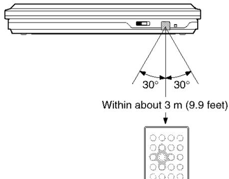
Distance: About 3 m (9.9 feet) from the front of the remote sensor
