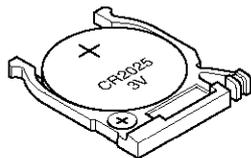
Keep the holder horizontal so that the battery does not fall through.
