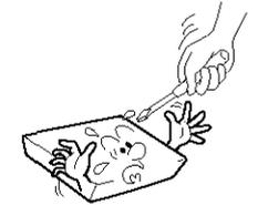
c) Never short-circuit the battery pack by either accidentally or intentionally bringing the terminals in contact with another metal object. This could cause personal injury or a fire, and could also damage the battery pack.
