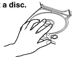
Place a disc with the playback side down, and push gently on the center of the disc to affix it to the spindle.
