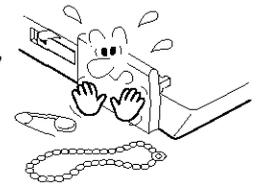
d) Never drive a nail into the battery pack. Never strike the battery pack with a hammer. Never step or tread on the battery pack.
