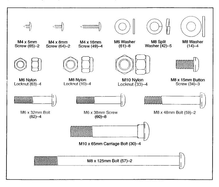
While another person lifts the front of the Frame (1) slightly, attach a Stabilizer (2) with two M10 x 65mm Carriage Bolts (30) and two M10 Nylon Locknuts (33).
