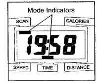
mode indicator will show which mode is currently displayed. Note: If you have selected a different mode, repeatedly press the Mode button to reselect the scan mode.
