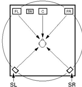
In this case the speakers should surround the listener from all sides to create a uniform sound field from 360°. Ideally the surround speakers should function as "point" sound sources in the same way as the front speakers.
