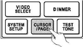
Press "CURSOR/PAGE" at the center of the bottom line on the "AV AMP's" "SETTING 3/5" page so that this part is displayed in half-tone dot mesh. Make the system setups by pushing the jog stick on the remote control unit forward and backward, left and right.
