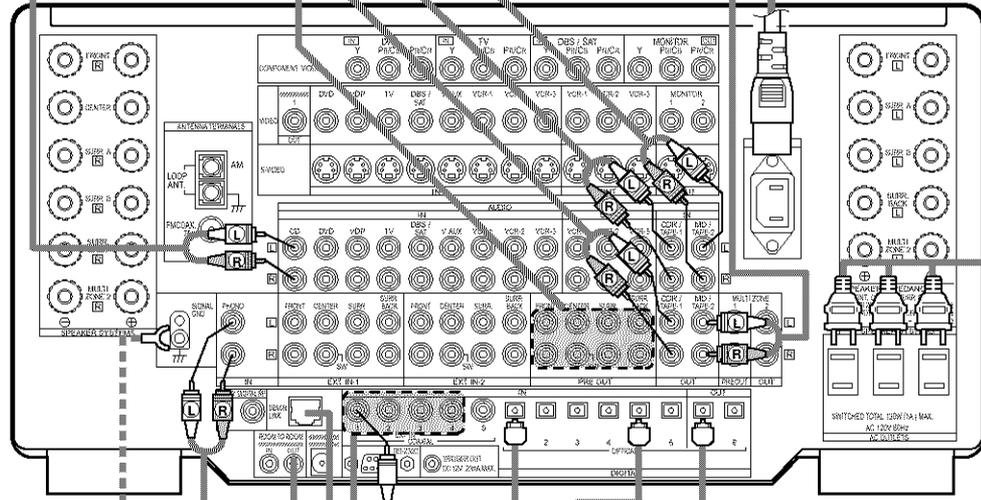
MD recorder, DAT deck or other component equipped with digital input/output jacks
