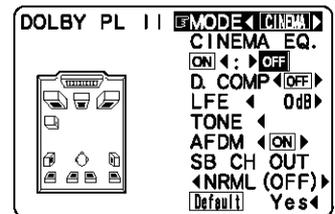
**5** Select the optimum mode for the source. Turn the FUNCTION knob and display “MODE CINEMA”, then turn the CONTROL knob and select the mode.
