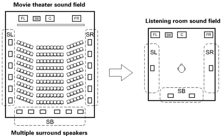
In this case it is important to achieve the same sense of expansion as in a movie theater with the surround channels. To do so, in some cases the number of surround speakers is increased (to four or eight) or speakers with bipolar or dipolar properties are used.
