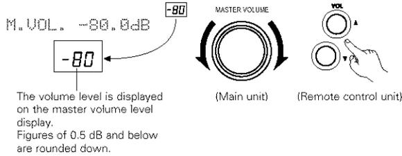
※ The volume can be adjusted within the range of -80 to 0 to 18 dB, in steps of 0.5 dB. However, when the channel level is set as described on page 24 or page 48, if the volume for any channel is set at +1 dB or greater, the volume cannot be adjusted up to 18 dB. (In this case the maximum volume adjustment range is "18 dB - (Maximum value of channel level)".)
