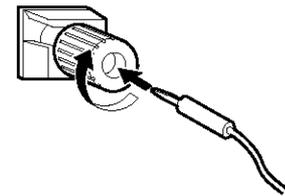
Turn clockwise to tighten, then insert the banana plug.
