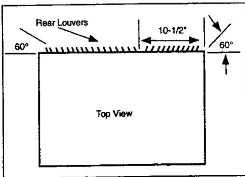
1. Redirect the louvers at the back of the wall sleeve as shown in the illustration. The use of pliers is recommended.
