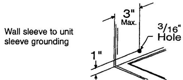
4. Prepare the wall sleeve for installation of the new unit per the following Brand instructions.
