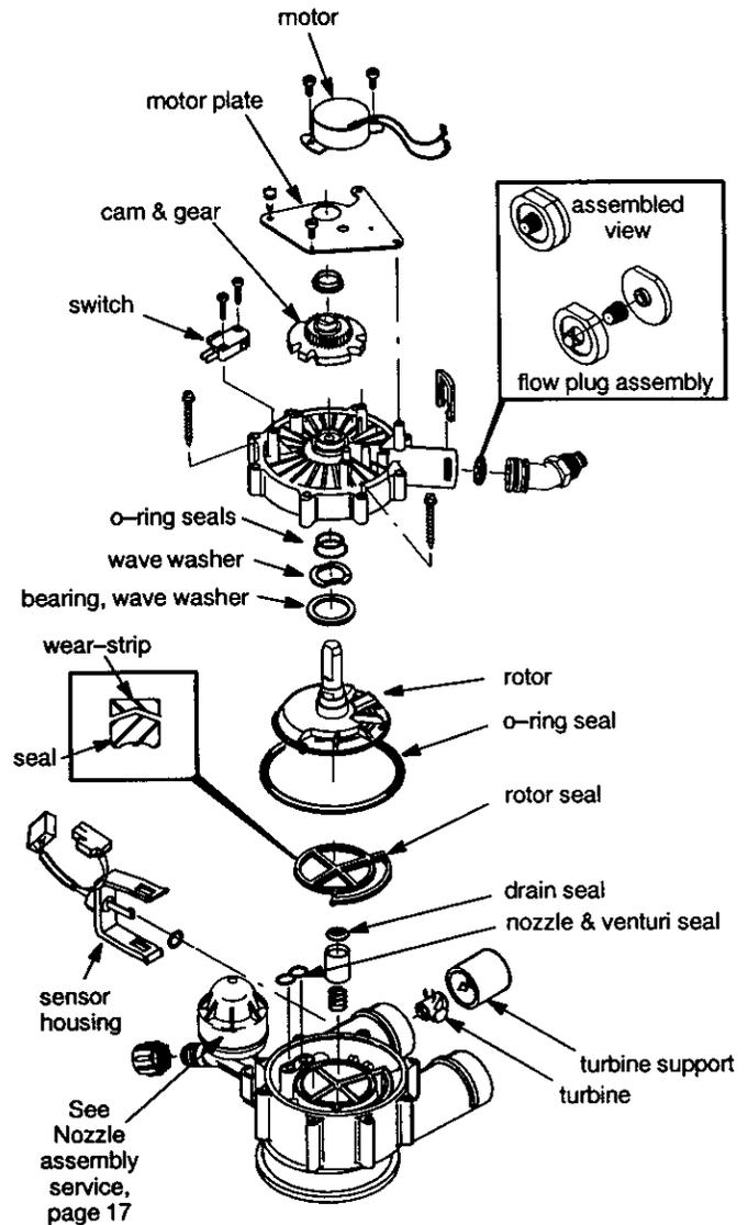
Lubricate the gear on the motor, and the valve cam gear with Molykote grease, or other high quality gear lubricant.
