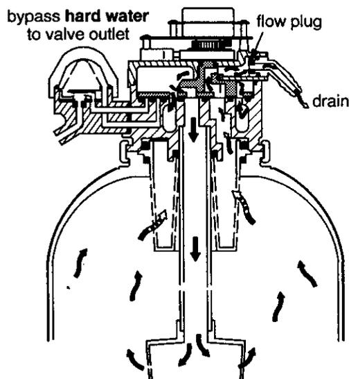
Timer/switch action again allows the motor to turn the rotor & disc to place the valve in BACKWASH, stopping water flow to the nozzle. Water is routed down and out the bottom distributor, up through the bed, and out the top distributor to the drain. The fast flow (controlled by a flow plug in the drain fitting) flushes dirt, sediments, iron deposits, remaining brine and hardness to the drain.
