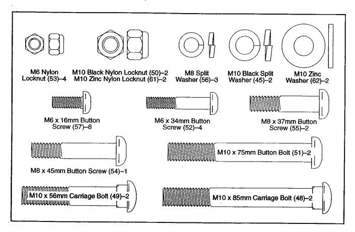
Identify the Front Stabilizer (2). Turn the Front Stabilizer so that the warning decal is in the position shown. While another person lifts the front of the Frame (1) slightly, attach the Front Stabilizer to the Frame with two M10 x 85mm Carriage Bolts (48) and two M10 Black Nylon Locknuts (50).
