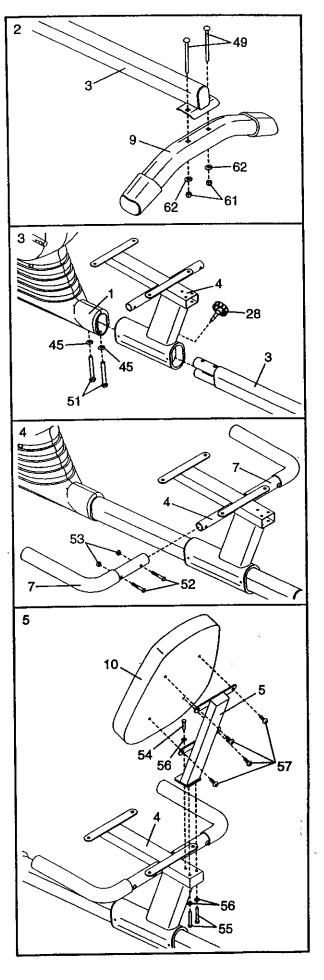
6. Attach the Seat (12) to the Seat Carriage (4) with four M6 x 16mm Button Screws (57).
