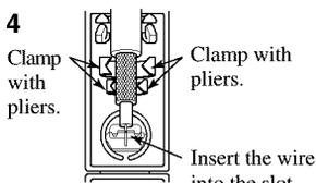
Insert the cable wire into the slot, and clamp it with pliers.
