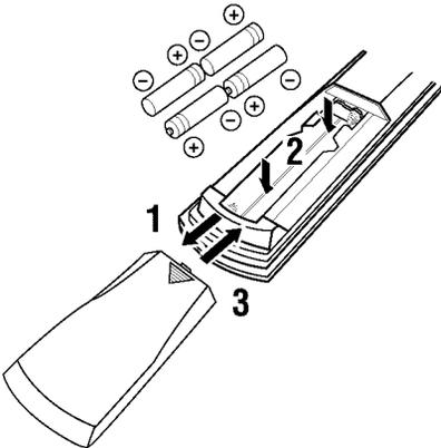
**1** Press the ▼ part and slide off the battery compartment cover.
