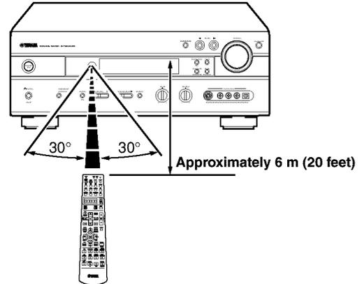
The remote control transmits a directional infrared beam. Be sure to aim the remote control directly at the remote control sensor on the main unit during operation.
