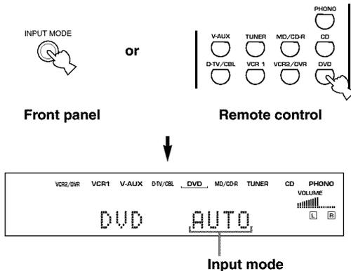
**AUTO:** In this mode, the input signal is selected automatically as follows:
