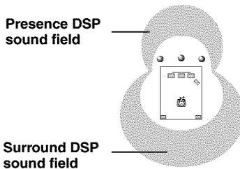
Most movie software has 4-channel (left, center, right, and surround) sound information encoded by Dolby Surround matrix processing and stored on the left and right tracks. These signals are processed by the Dolby Pro Logic decoder. The MOVIE THEATER programs are designed to recreate the spaciousness and delicate nuances of sound that tend to be lost in the encoding and decoding processes.
