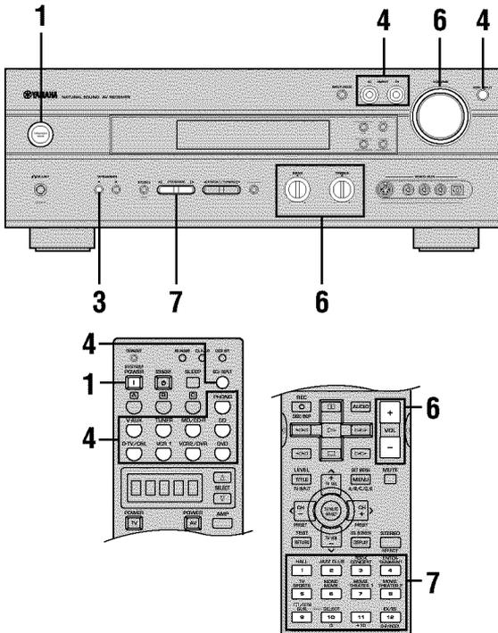
**1** Press **STANDBY/ON** (**SYSTEM POWER** on the remote control) to turn on the power.
