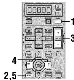
**1** Press **AMP** to select the **AMP** mode. “AMP” appears in the display window on the remote control.
