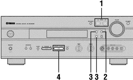
**1** Press INPUT  $\triangleleft/\triangleright$  (TUNER on the remote control) to select TUNER as the input source.
