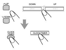
**4** Press UP or DOWN to select the timer mode (Daily Timer or Recording Timer) and the source to play, then press CLOCK/TIMER.
