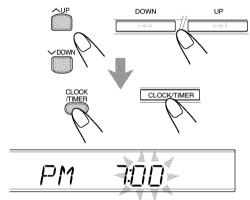
**3** Press UP or DOWN to adjust the minute, then press CLOCK/TIMER.
