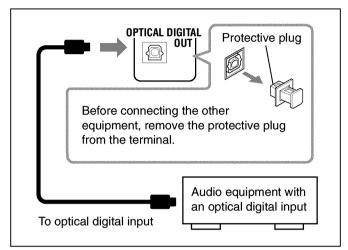
Connect an optical digital cord (not supplied) between the optical digital input terminal on the other equipment and the OPTICAL DIGITAL OUT terminal.
