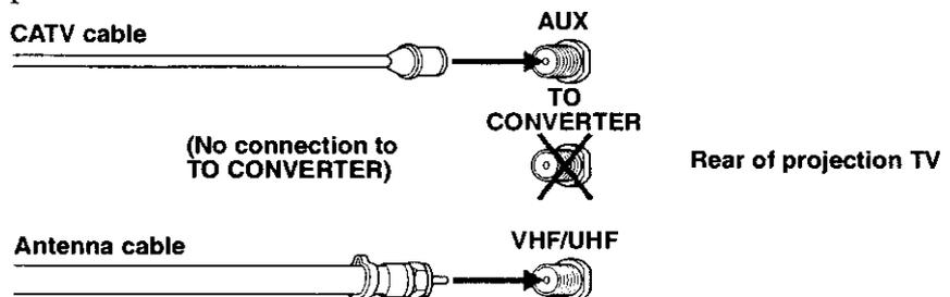
Select CABLE or antenna (ANT) mode by pressing ANT on the remote control.
