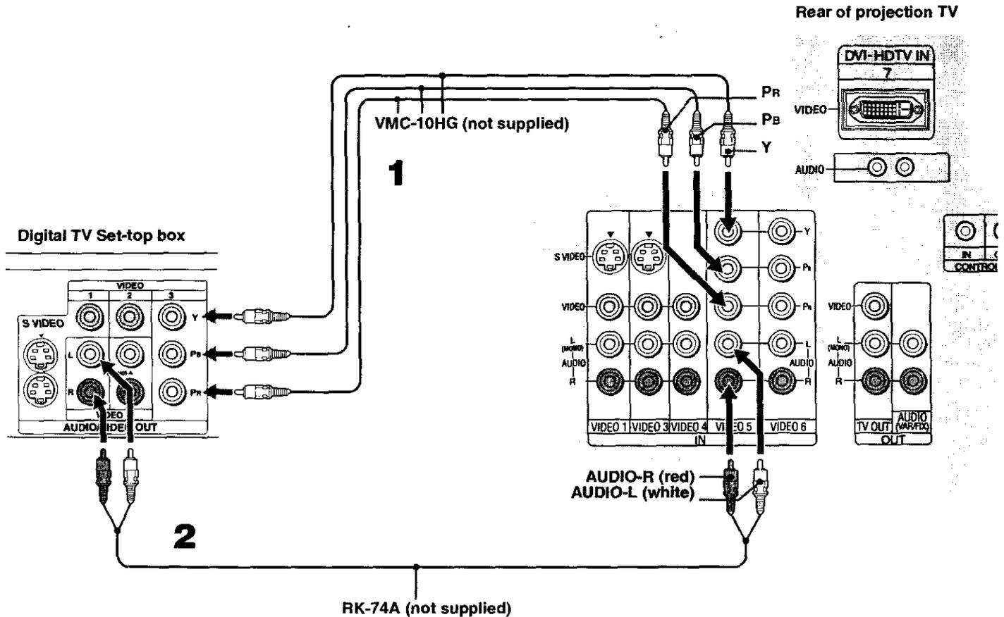
**⚠** You cannot record the signal from any equipment connected into the Y, Pb and Pr connectors.
