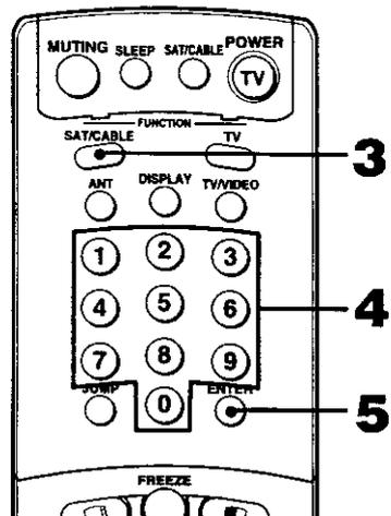
From the "Manufacturer's Codes" listed on page 70, select the three-digit code number for the manufacturer's code for your component. If more than one code number is listed, start with the number listed first. Use the code number to complete the following procedure.
