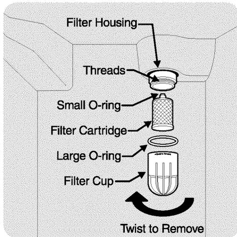
Order new filter cartridges through the dealer where you bought the refrigerator, or contact the *Consumer Assistance Center* at 1-800-944-9044. It might be good to order some filter cartridges when you first install your refrigerator. Be sure to ask for the *RG-100 PureSource™\** replacement cartridge.
