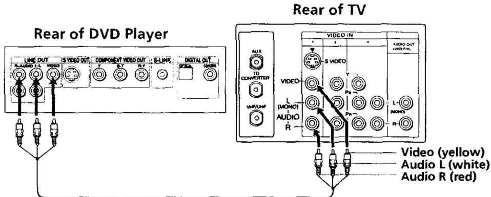
For better picture quality, use S VIDEO instead of the yellow video cable. S VIDEO does not provide sound; you still must connect the audio cables.
