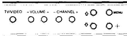
The front Audio/Video panel controls allows you to access the menu without the remote control.
