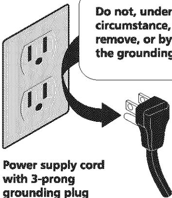
Do not, under any circumstance, cut, remove, or bypass the grounding prong.
