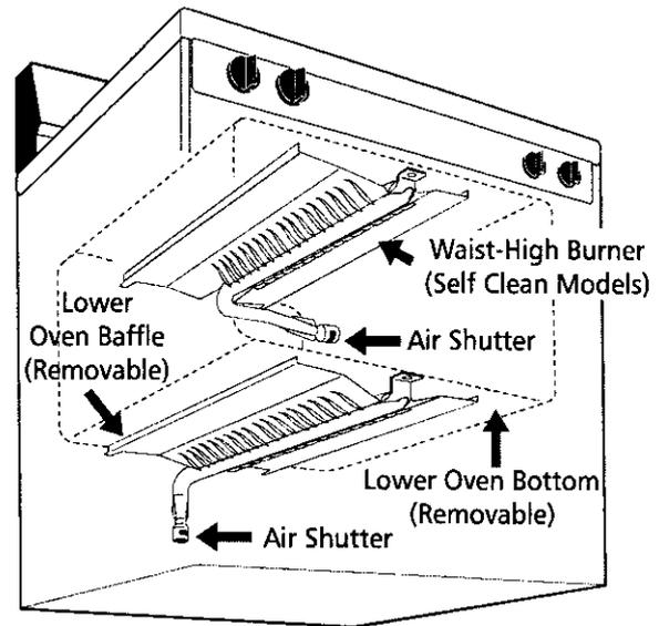
If the flame is yellow in color, increase air shutter opening size. (See "2" in illustration below.) If the flame is a distinct blue, reduce the air shutter opening size.
