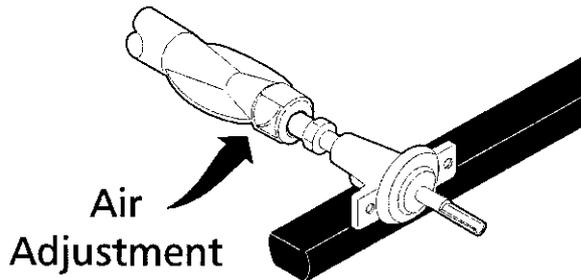
If the air is properly adjusted, the flame will be steady, relatively quiet, and have approximately 1/2" sharp blue cone. (Usually about the center of air shutter's adjustment.)
