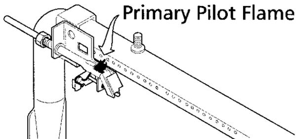
After 20-40 seconds, the main oven burner should ignite and burn until the oven temperature has reached 300°F. At that time, the oven pilot should get smaller, moving up away from the metal bulb which will turn off the main oven burner after 20-40 seconds.
