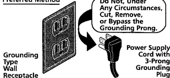
Where a standard two-prong wall receptacle is encountered, it is the personal responsibility and obligation of the customer to have it replaced with a properly grounded three-prong wall receptacle.
