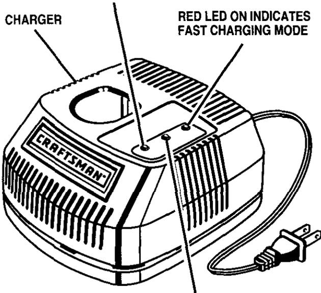
GREEN LED ON AFTER FAST CHARGING CYCLE, INDICATES FULLY CHARGED BATTERY PACK AND IN TRICKLE CHARGE MODE.
