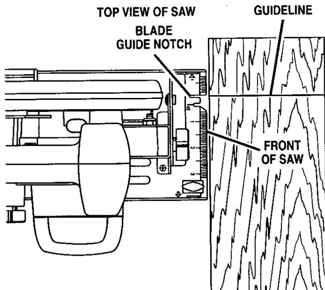
ALIGN OUTER BLADE GUIDE NOTCH ON SAW BASE WITH LINE OF CUT AS SHOWN WHEN MAKING CROSS CUTS OR RIP CUTS
