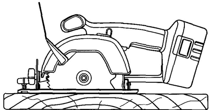
BLADE EXPOSED ON UNDERSIDE OF WORKPIECE
