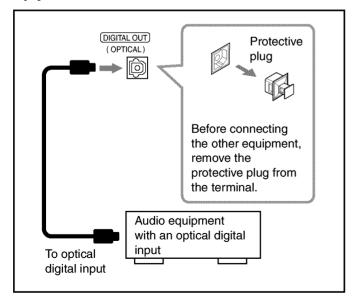
Connect an optical digital cord (not supplied) between the optical digital input terminal on the other equipment and the DIGITAL OUT [OPTICAL] terminal.
