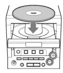
4 Press ▲ OPEN/CLOSE to close the disc compartment. The total number of tracks and the playing time of the disc appear on the display.
