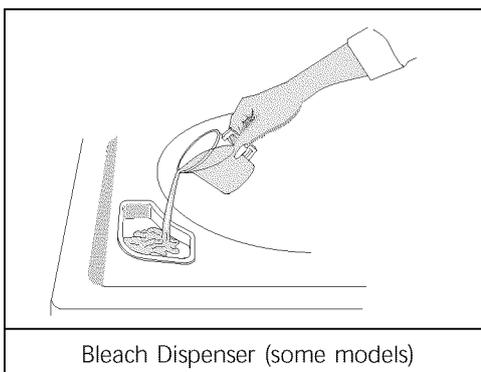
**For models without a bleach dispenser**, dilute the recommended amount of liquid chlorine bleach in 1 quart (.95 L) water. Add it to wash water after a few minutes of agitation. **Do not pour bleach directly on wash load.**
