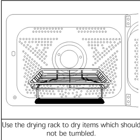
Use the drying rack to dry items which should not be tumbled.
