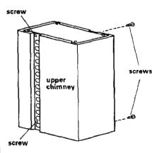
Remove the four screws on the upper chimney and disassemble chimney pieces from support frame.
