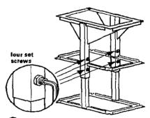
Determine the height of the canopy. The range hood requires at least 24" (61 cm) of clearance between bottom of range hood canopy and cooking surface.
