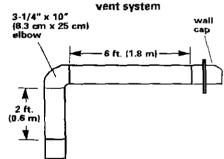
Maximum length = 35 ft. (10.7 m) 1 — 90° elbow = 5 ft. (1.5 m) 8 ft. (2.4 m) straight = 8 ft. (2.4 m) 1 — wall cap = 0 ft. (0 m) Length of 3-1/4" x 10" (8.3 cm x 25 cm) system = 13 ft. (4 m)
