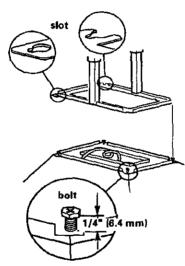
11. Loosen four bolts located next to exhaust opening so that there is approximately 1/4" (6.4 mm) space between bolt head and canopy. Lift canopy and insert bolts into slots in support system frame. Tighten bolts to support system frame and canopy.
