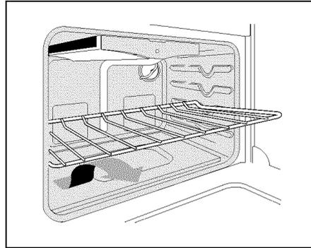
**To remove an oven rack**, pull the rack forward until it stops. Lift up front of rack and slide out. **To replace an oven rack**, fit the rack onto the guides on the oven walls. Tilt the front of the rack upward and slide the rack back into place.
