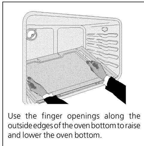
Use the finger openings along the outside edges of the oven bottom to raise and lower the oven bottom.
