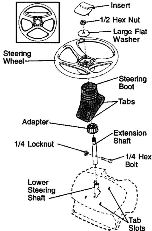
6. Assemble large flat washer, 1/2 hex nut and tighten securely.
