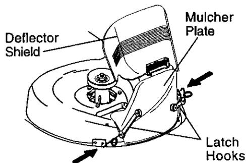
**CAUTION:** Do not remove deflector shield from mower. Raise and hold shield when attaching mulcher plate and allow it to rest on plate while in operation.
