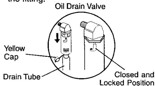
3. Unlock drain valve by pushing upward slightly and turning counterclockwise.
