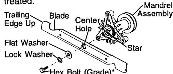
\*A Grade 8 heat treated bolt can be identified by six lines on the bolt head.
