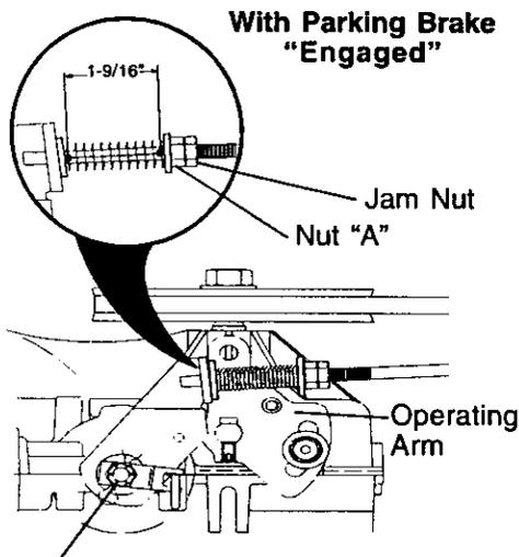
Do Not touch this nut. If further brake adjustment is necessary contact a Sears or other qualified service center.
