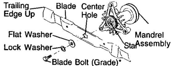
\*A Grade 8 heat treated bolt can be identified by six lines on the bolt head.
