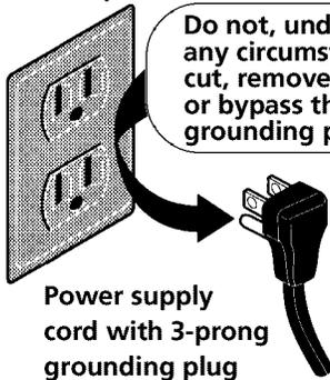
Power supply cord with 3-prong grounding plug
