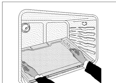
Use the finger openings along the outside edges of the oven bottom to raise and lower the oven bottom.
