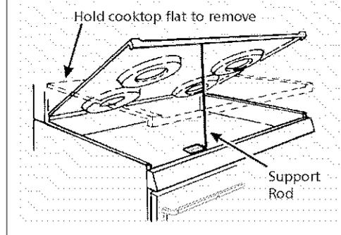
**⚠ WARNING** **DO NOT** turn the burners on when the cooktop is raised for cleaning. Be sure that the top is completely lowered and securely in place before turning on the burners.
