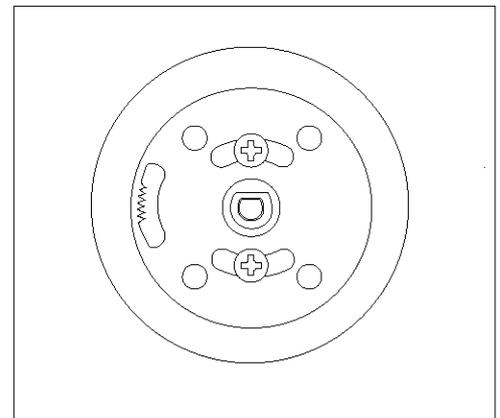
**Note:** Once an adjustment is made, the OFF position will vary from the reference mark on the backguard depending on the amount of adjustment.
